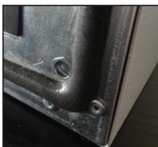
Polyurethane gasket machinery applied
