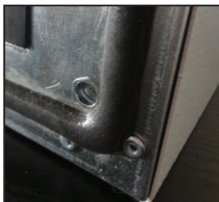
Polyurethane gasket machinery applied
