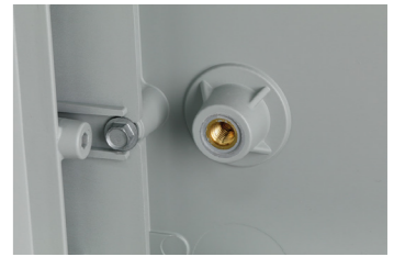
INSERTS WITH M10 THREAD BURIED IN THE BASE PANEL DURING THE MOULDING PHASE ALLOW BOTTOM PLATES TO BE APPLIED.
